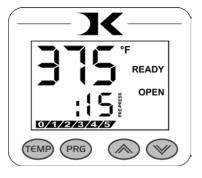
the main timer for 20. When the operator closes the press, the 5-sec time counts down. When the operator opens the press, the time setting switches to 20 seconds.
